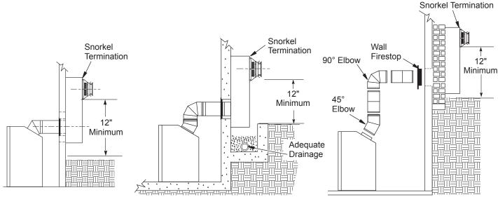
Figure 16 - Snorkel Termination Configurations for Below Ground Installation
